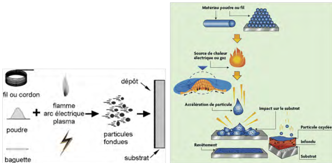
FIGURE 2.18 – Principe de la projection thermique
