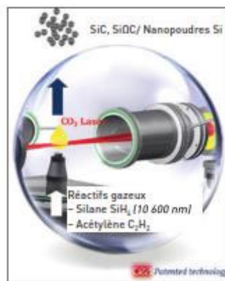
Figure 2: Operating principle of laser pyrolysis, allowing atoms to be obtained from gaseous molecules.
