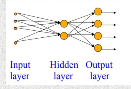
2-layer or 1-hidden layer *fully connected* network
