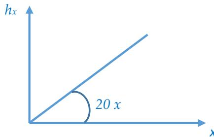
$$\bar{h}_x = \frac{1}{L} \int_0^L h_x dx = \frac{1}{5} \int_0^5 20 x dx = \frac{20}{5} \frac{1}{2} x^2 \Big|_0^5 = 50 \left[ \frac{\text{W}}{\text{m}^2\text{K}} \right]$$
