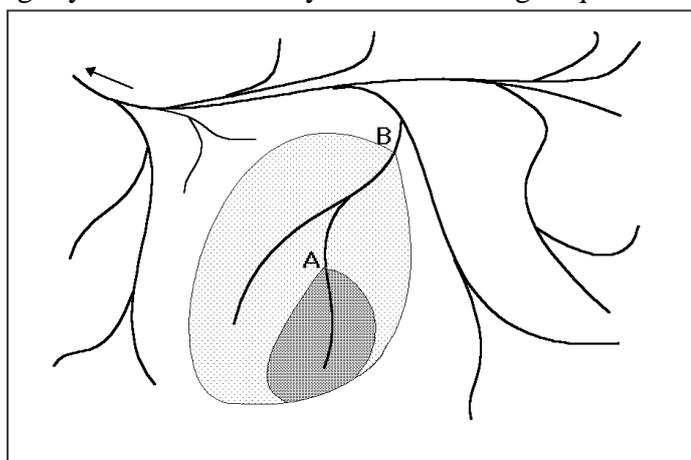
Fig. 1.4 The catchment area increases as the control point moves down stream
