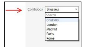
In computer science, a combined box (in English combo-box or combo box) is an element of graphic interface which brings together a text zone and an dropdown. This element is commonly used by Web sites and software.
