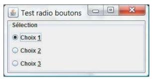
A radio button (in English radio button) is a visual element of graphical interfaces always used in groups (two radio buttons at least). The user must choose one, and only one, option from several possible ones.
