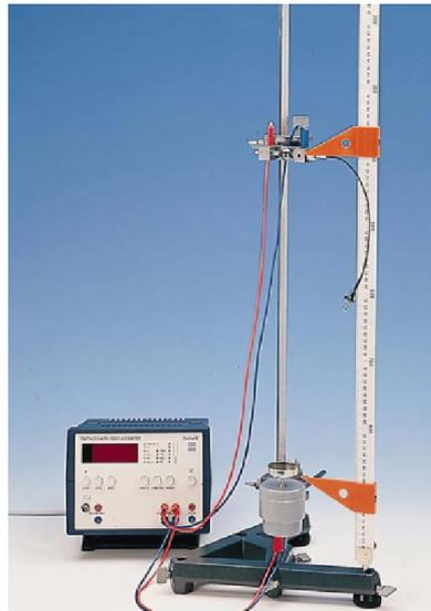
Figure 3.1 Montage essai chute
