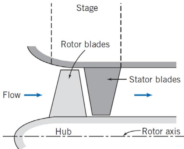
(a) Axial-flow compressor stage
