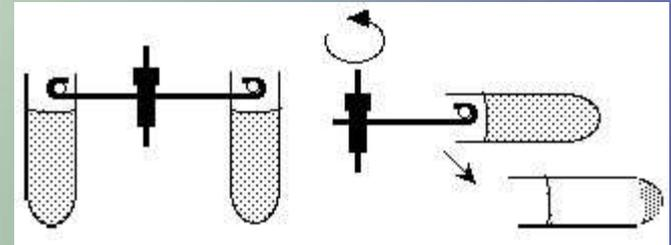
**Longer distance of travel may allow better separation, such as in density gradient centrifugation. Easier to withdraw supernatant without disturbing pellet.**
