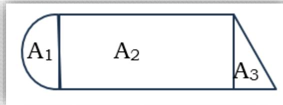
$$x_g = \frac{\sum_{i=1}^n x_i A_i}{\sum_{i=1}^n A_i} \quad y_g = \frac{\sum_{i=1}^n y_i A_i}{\sum_{i=1}^n A_i}$$
