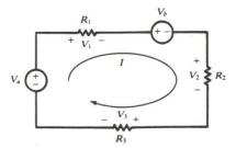
b- KVL is used to combine the voltage sources present in series.
