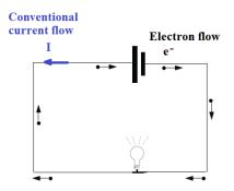
An electron flowing from – to + gives rise to the same "conventional current" as a proton flowing from + to -
