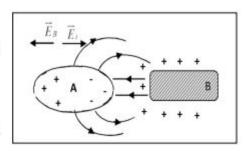
to the creation of an electric field inside the conductor. Electrostatic influence divides the charge inside the conductor. This phenomenon is called **partial influence**.
