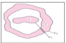
see that its potential varies so that the Q/V ratio remains constant. This ratio is called the conductor capacity and is denoted C (in Farad)
