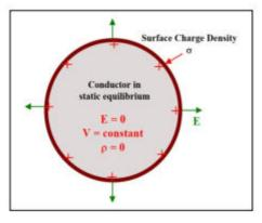
the surface charge density (i.e. charge per unit area) and the net charge on the conductor is  $Q = \int\limits_{Surface} \sigma dS \ .$
