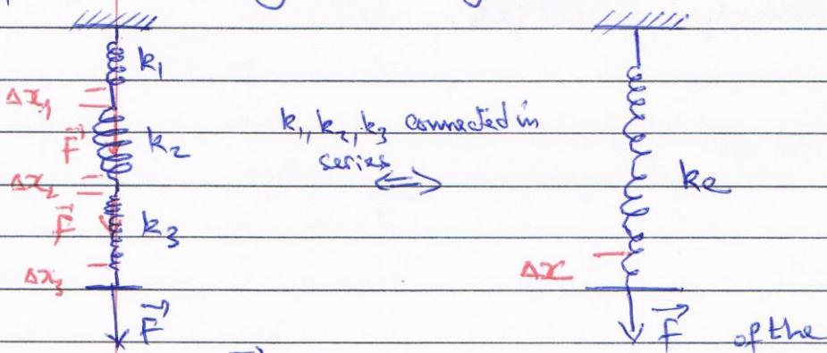
The same force  $\vec{F}$  is transmitted to each springs  $k_1, k_2$  et  $k_3$ , in series and consequently, the force  $\vec{F}$  causes different elongations;  $\Delta x_1, \Delta x_2$  and  $\Delta x_3, \dots$  successively. Then we have:
