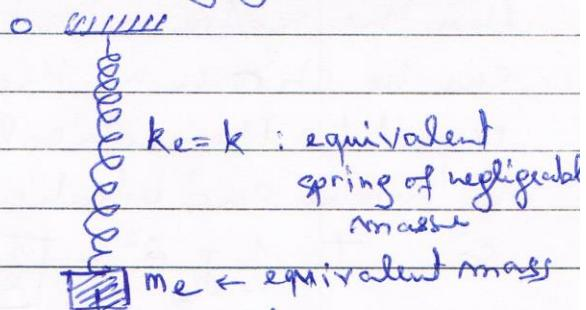
We take an infinitesimal element  $dl$  from the real spring, which is around of a certain point  $s$ , which is located at a distance  $l$  from the suspension point of the spring (point  $O$ )
