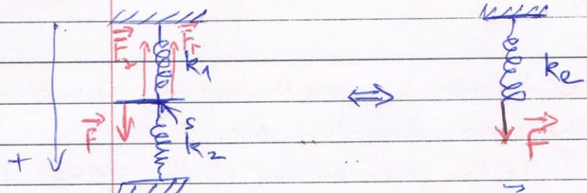
under the influence of the force  $\vec{F}$  the point \$S\$ is moved by  $\Delta x$  downward. Then the spring  $k_1$  is elongated by  $\Delta x$  and  $k_e$  is compressed by  $\Delta x$
