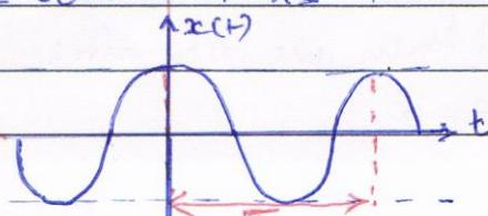
$$x(t) = x_0 \cos\left(\sqrt{\frac{k}{m}} t\right) \Rightarrow T_0 = \frac{2\pi}{\omega_0} = 2\pi \sqrt{\frac{m}{k}}$$
