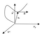
$$\vec{a}(t) = \lim_{\Delta t \to 0} \frac{\Delta \vec{v}}{\Delta t} = \frac{d\vec{v}}{dt} = \frac{dv_x}{dt}\vec{i} + \frac{dv_y}{dt}\vec{j} + \frac{dv_z}{dt}\vec{k}$$
