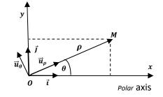
x: is the projection of  $\overline{OM}$  on the direction  $\vec{i}$
