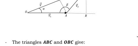
$$\begin{cases} \sin(\alpha) = \frac{BC}{OC} \\ \sin(\pi - \beta) = \frac{BC}{AC} \end{cases} \Rightarrow OC. \sin(\alpha) = AC. \sin(\beta) \Rightarrow \frac{|\vec{V}|}{\sin(\beta)} = \frac{|\vec{V}_2|}{\sin(\alpha)} \\ - \text{ The triangles } OAD \text{ and give:} ACD \end{cases} \Rightarrow \frac{|\vec{V}|}{\sin(\beta)} = \frac{|\vec{V}_2|}{\sin(\beta)} = \frac{|\vec{V}_2|}{\sin(\beta)} = \frac{|\vec{V}_2|}{\sin(\beta)} = \frac{|\vec{V}_1|}{\sin(\gamma)} \end{cases}$$
