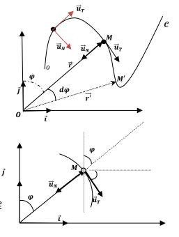
$$\Rightarrow \begin{cases} \vec{u}_T = \frac{d\vec{u}_T}{dt} = -\frac{d\varphi}{dt} (\sin\varphi \,\vec{i} + \cos\varphi \,\vec{j}) = \dot{\varphi} \,\vec{u}_N \\ \vec{u}_N = \frac{d\vec{u}_N}{dt} = -\frac{d\varphi}{dt} (\cos\varphi \,\vec{i} - \sin\varphi \,\vec{j}) = -\dot{\varphi} \,\vec{u}_T \end{cases}$$
