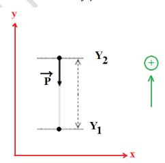
$$W_{y1\to y2} = -\int_{y_1}^{y_2} mg \ dy = - mg \ (y_2-y_1)$$
