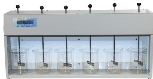
Figure 10 : Jar Tests
