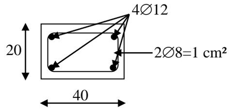
$$\frac{A_l \cdot f_e}{S_t \cdot \gamma_s} = \frac{M_T}{2 \cdot \Omega} \quad \Rightarrow \quad S_t = \frac{A_l \cdot f_e \cdot 2 \Omega}{M_T \cdot \gamma_s} = \frac{0,0001 \times 235 \times 2 \times 0,061129}{0,01 \times 1,15} = 25 \text{ cm}$$
