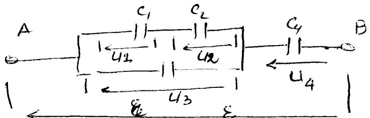
$$\text{l'équation } \textcircled{2}. \quad Q_3 + Q_2 = Q_3 + Q_1 = Q \Rightarrow Q_1 = Q - Q_3 = (89,5 - 63,2) \cdot 10^{-6}$$
