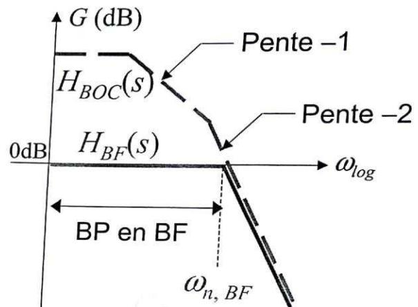
Relation temps de montée-BP ( $t_m = 2,2/\omega_{c,BF}$ )  $\omega_{n,BF} = \omega_{n,0} \sqrt{1+K_0} \approx \omega_{c0}$
