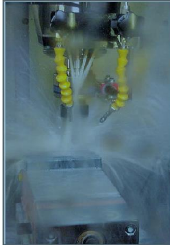
Drilling with the rotating system Type 9125A...
