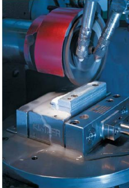
Lateral grinding of silicon workpieces with dynamometer Type 9256C1
