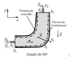
$$-p_{1}S_{1}\vec{n}_{1} + p_{2}S_{2}\vec{n}_{2} + \iint_{S_{l}} -p\vec{n}_{l}dS + m\vec{g} = \rho(Q_{2}\vec{U}_{2} - Q_{1}\vec{U}_{1})$$
