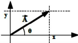
$$\vec{A} = x\vec{i} + y\vec{j}, \quad \|\vec{A}\| = \sqrt{x^2 + y^2} \quad \begin{cases} x = \|\vec{A}\| \cos \theta \\ y = \|\vec{A}\| \sin \theta \end{cases} \text{ et } \tan \theta = \frac{y}{x}$$
