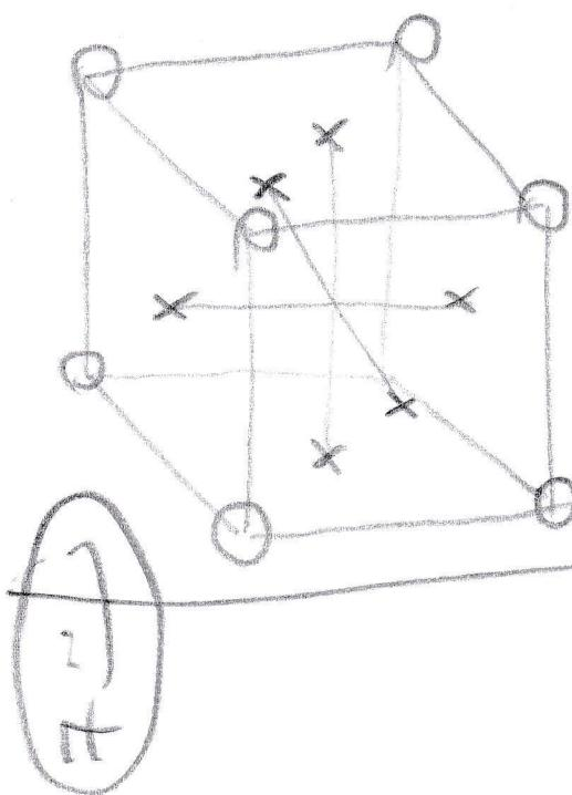
$$Z_{\text{Cu-Au}} = 4 \\ Z_{\text{Cu-Cu}} = 8 \\ R_{\frac{1}{2}} = \frac{\sqrt{2}}{2} a.$$
