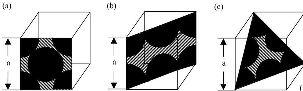
area intersected by the (1 0 0) plane and the FCC unit cell is  $a^2$  while the number of atoms contained is:
