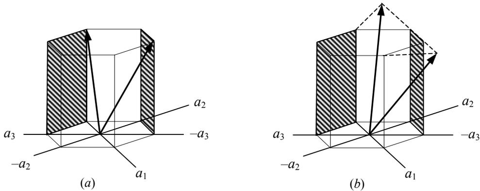
For Fig. P3.67(a), the Miller-Bravais direction indices indicated are  $[\bar{2} 1 1 1]$  and  $[1 1 \bar{2} 1]$ . Those associated with Fig. P3.67(b) are  $[\bar{1} 1 0 1]$  and  $[1 0 \bar{1} 1]$ .
