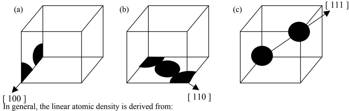
$$\rho_l = \frac{\text{no. of atomic diam. intersected by selected length of direction line}}{\text{selected length of line}}$$
