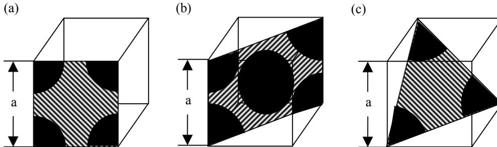
To calculate the density, the planar area and the number of atoms contained in that area must first be determined.
