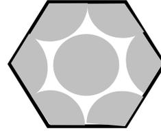
$$\text{Selected Area} = (6 \text{ triangles}) \times (\text{equilateral triangle area}) = 6 \left( \frac{1}{2} a \right) \left( \frac{\sqrt{3}}{2} a \right) = \frac{3\sqrt{3}}{2} a^2$$
