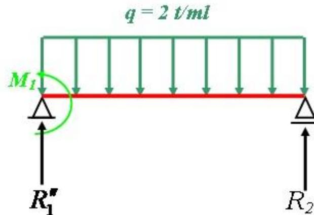
$$R_0 = -2.015 \text{ t}; \quad R_1 = 12.187 \text{ t}; \quad R_2 = 4.828 \text{ t}$$
