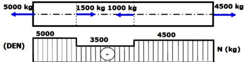
$$\begin{aligned} \Delta L &= \int_0^L \frac{N}{ES} dx = \int_0^{L_1} \frac{N_1}{ES_1} dx + \int_{L_1}^{L_1+L_2} \frac{N_2}{ES_2} dx + \int_{L_1+L_2}^L \frac{N_3}{ES_3} dx \\ &= \frac{N_1 L_1}{ES_1} + \frac{N_2 L_2}{ES_2} + \frac{N_3 L_3}{ES_3} \\ &= \frac{1}{E} \sum_{i=1}^3 \frac{N_i L_i}{S_i} \end{aligned}$$
