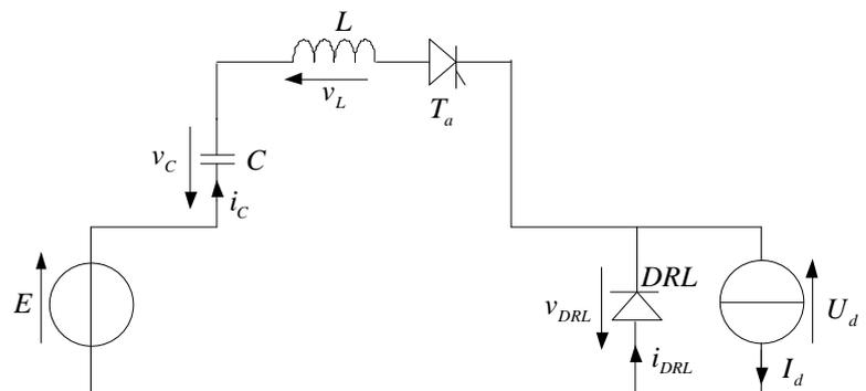
Or  $v_L = L \frac{di_C}{dt}$  et  $i_C = C \frac{dv_C}{dt} \Rightarrow v_L = LC \frac{d^2 v_C}{dt^2}$
