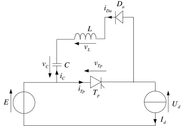
$$\text{Or } v_L = L \frac{di_C}{dt} \text{ et } i_C = C \frac{dv_C}{dt} \Rightarrow v_L = LC \frac{d^2 v_C}{dt^2}$$
