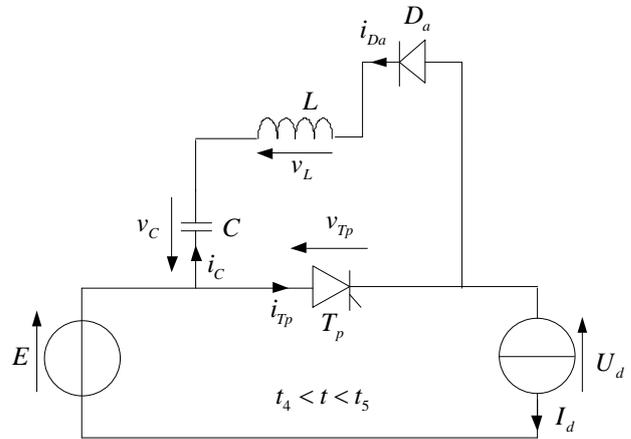
Or  $v_L = L \frac{di_c}{dt}$  et  $i_c = C \frac{dv_C}{dt} \Rightarrow v_L = LC \frac{d^2v_C}{dt^2}$
