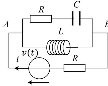
$$Z_{AB} = \frac{jL\omega \left( R + \frac{1}{jC\omega} \right)}{R + jL\omega + \frac{1}{jC\omega}} = \frac{jL\omega(1 + jRC\omega)}{(1 - LC\omega^2) + jRC\omega}$$
