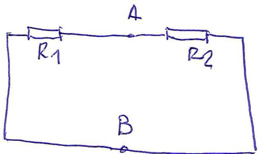
$$R_{Th} = \frac{R_1 R_2}{R_1 + R_2}$$
