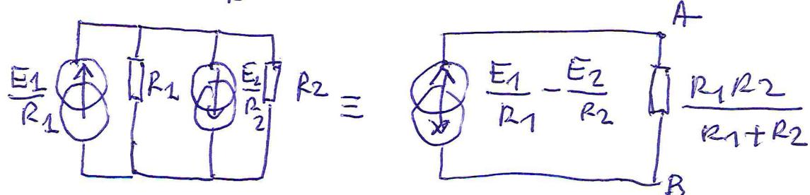
$$V_{AB} = \left( \frac{E_1}{R_1} - \frac{E_2}{R_2} \right) \frac{R_1 R_2}{R_1 + R_2}$$
