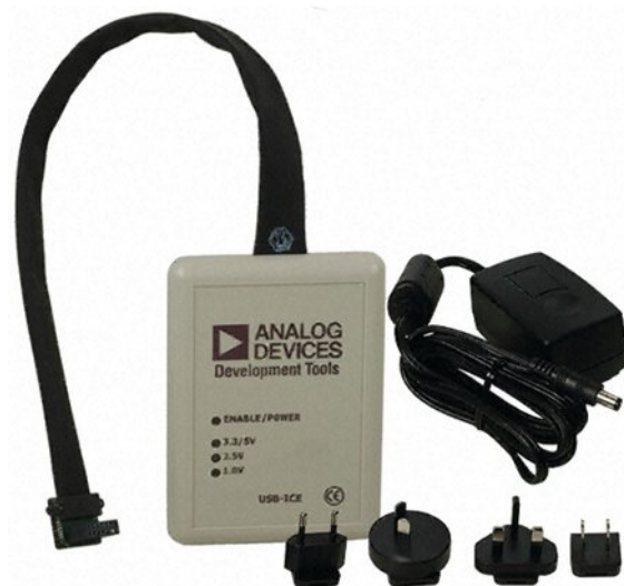
Figure 4.3 : Emulateur USB haute performance 1,5Mo/s
