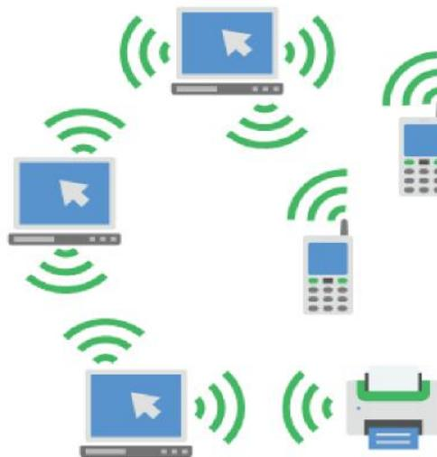
FIGURE.11. RESEAU AUTONOME WI-FI AD-HOC
