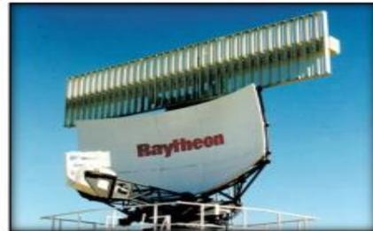
*ASR-10SS PSR with co-mounted MSSR*
